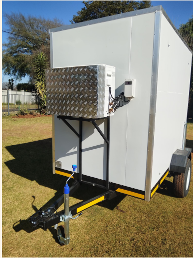
External refrigeration condensing unit
